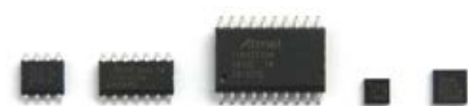
Slika 1: Izbor novih ATtiny čipov: SOIC ATtiny412, ATtiny1614 in ATtiny3216; QFN ATtiny1616 in ATtiny3217. (fotografija: technoblogy.com)
